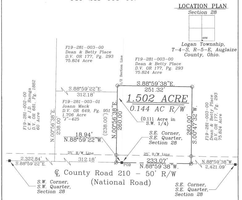
Basis of Bearing is the South Line of the Southeast Quarter of Section 28 and the centerline of C.R. 210 as N.88°59'38"W. based on Ohio State Plane-North Coordinate System NAD-83 (2011).
