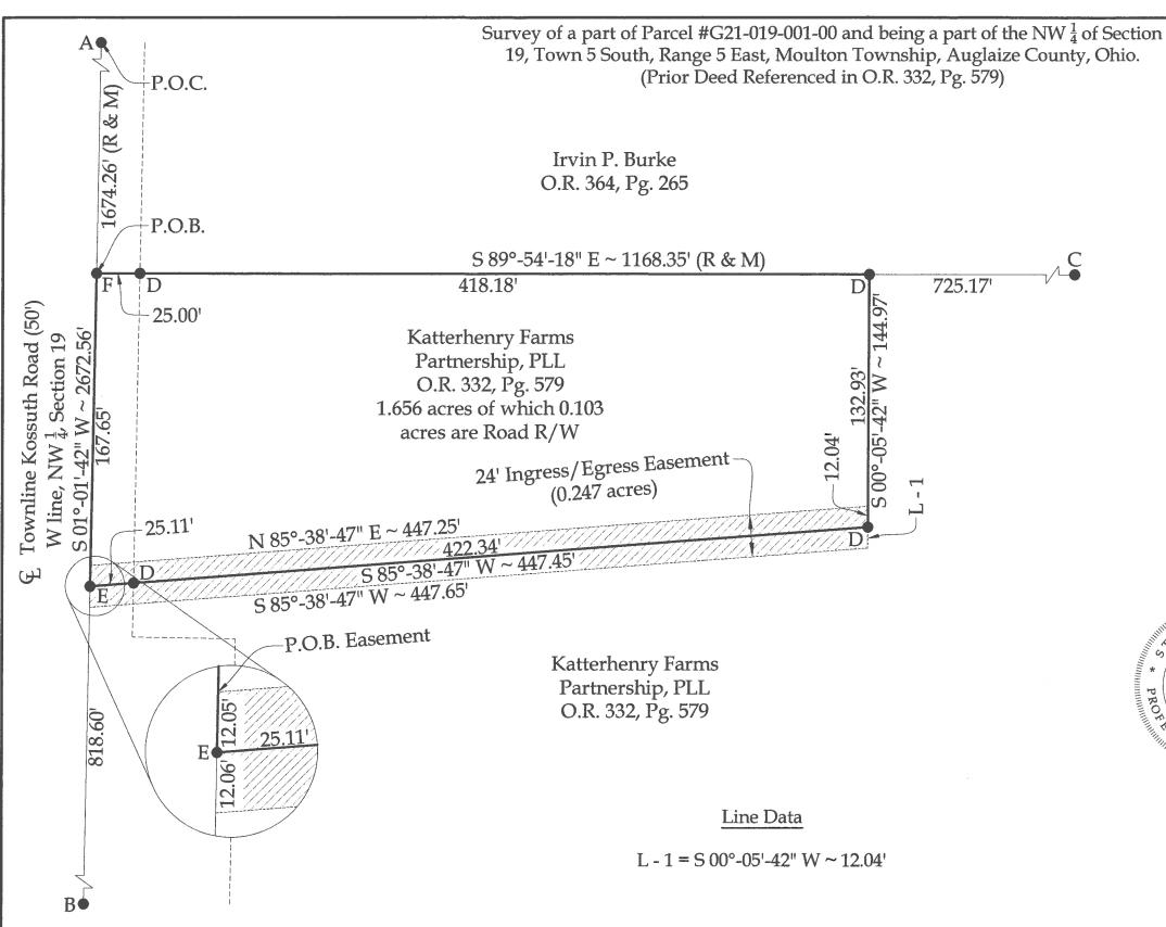
BASIS OF BEARINGS: The system of bearings for this plat and legal description is based on the Ohio State Plane - North Coordinate System NAD 83 (2011).
