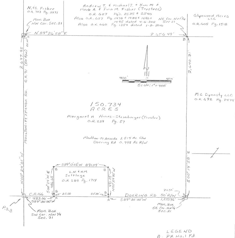
This plat represents a field survey performed in October,2020. All bearings refer to the south line of the northwest quarter of Section 21 as being S 89° 30' 00" W
