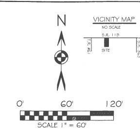
BASIS OF BEARING: BEARINGS ARE BASED ON THE OHIO DEPARTMENT OF TRANSPORTATION V.R.S. NAD 83(201 | ADJ.) OHIO STATE PLANE ZONE 3401.
