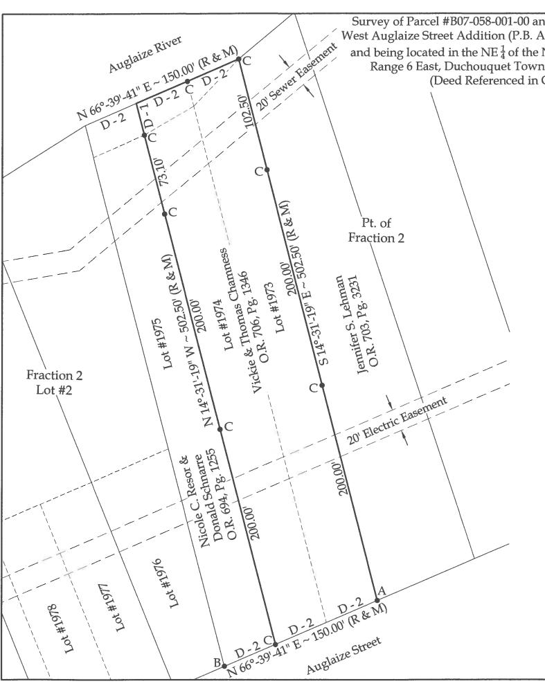
Survey of Parcel #B07-058-001-00 and being Lots #1973 & 1974 of the West Auglaize Street Addition (P.B. A, Pg. 13) in the City of Wapakoneta and being located in the NE  $\frac{1}{4}$  of the NE  $\frac{1}{4}$  of Section 31, Town 5 South, Range 6 East, Duchouquet Township, Auglaize County, Ohio. (Deed Referenced in O.R. 706, Pg. 1346)
