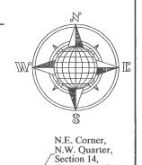
Basis of Bearing is the South line of the Northwest Quarter of Section 14, and the centerline of Gutman Road as N.88º46'24"W. from the Ohio State Plane-North Coordinate System NAD83 (2011).
