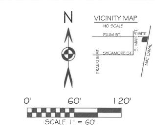
BASIS OF BEARING: BEARINGS ARE OHIO STATE PLANE NORTH ZONE, 3401, NAD 83, GRID DISTANCES SHOWN ARE GROUND.
