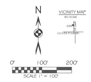
BASIS OF BEARING: BEARINGS ARE OHIO STATE PLANE NORTH ZONE, 3401, NAD 83, GRID DISTANCES SHOWN ARE GROUND.
