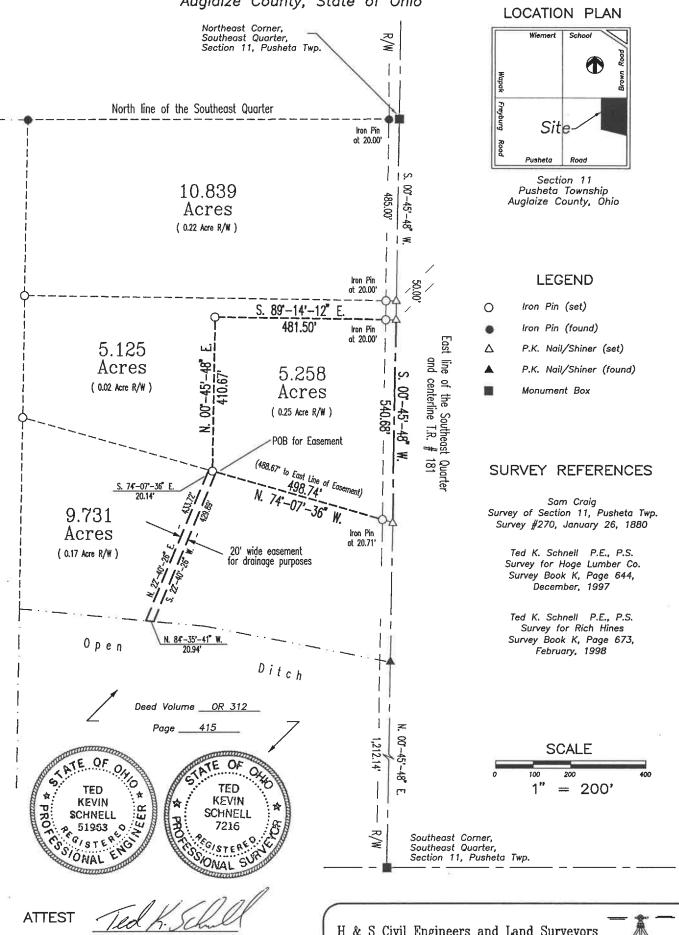
The Basis of Bearings used for this survey were determined from the Auglaize County Engineer's Global Positioning Survey of 1994. H & S Civil Engineers and Land Surveyors
