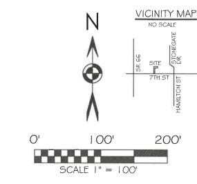
BASIS OF BEARING: BEARINGS & COORDINATES ARE OHIO STATE PLANE NORTH ZONE, 3401, NAD 83 (2011ADJ.), GRID. DISTANCES SHOWN ARE GROUND.
