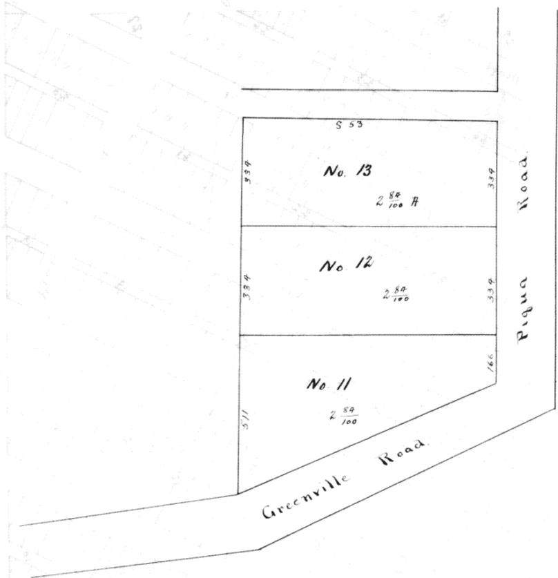
This Addition of Out Lots is situate immediately east and adjoining the former lots known on the record of Mercer County, as the Out Lots of Mitchell in the North West quarter of Section ten, town six south, range four east. The length of the line and dimensions are marked on the plat. The alley on the north is 33 feet wide.
