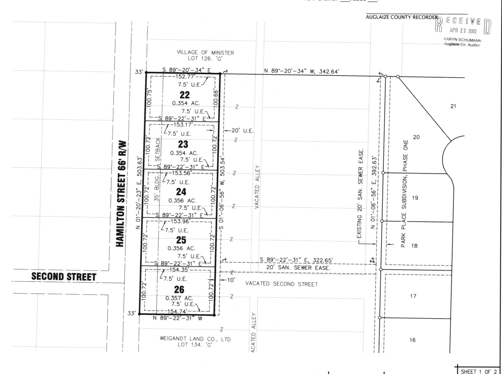
A 5/8"x 30" REBAR WITH CAP TO BE SET AT ALL LOT CORNERS AFTER CONSTRUCTION OF STREETS AND UTILITIES. Steven E. Bowers 5005-10-40
