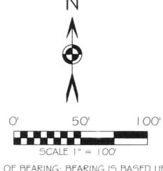
BASIS OF BEARING: BEARING IS BASED UPON THE CENTERLINE OF SR 274\MONROE STREET AND BEING N 86°03'58" E AS PER PLAT "GER-15-27" FILED IN THE AUGLAIZE COUNTY TAX MAP OFFICE.
